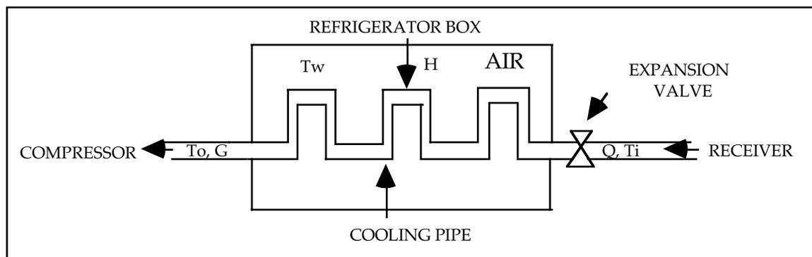
Figure 5. Evaporator (source from [Iwasaki 86]).
